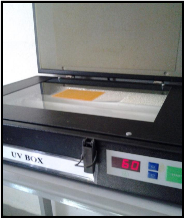
Figure 3.5 : Print circuit to the UV board
