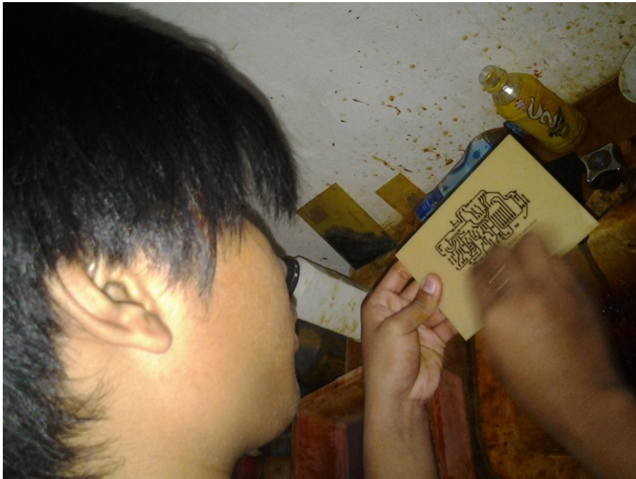
Figure 3.9 : Process to take out the green layer and leave the copper
