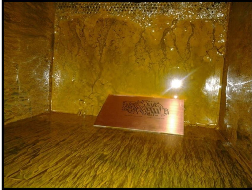
Figure 3.7 : Process automatically to take out the copper that un use
